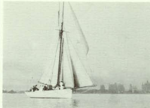
The sloop Merle , under sail, carrying—Main, Staysail, Jib, Jib Topsail and Club Topsail.
